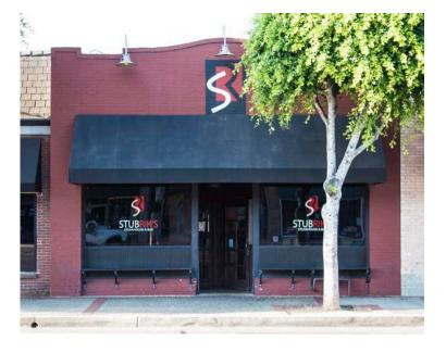
This one-story brick building is typical of the commercial buildings constructed during the 1920s, of which many were an imitation of the wood-framed structure that they replaced. The characteristic features are evident in this example: a compact rectangular shape, an unpretentious storefront design topped with transom windows, and a flat roof with decorative parapet. The 3,200-sq.-ft. building virtually covers the 25-ft.-wide lot.
